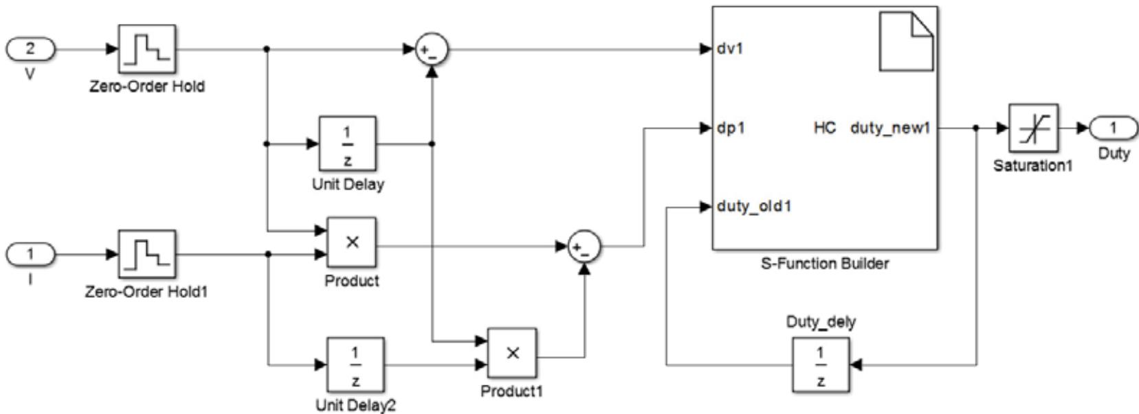
The diagram of MPPT for hill climbing method in Matlab
