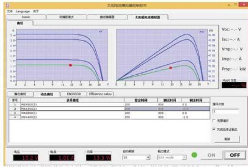
The solar array emulator PVS1000 Series (a) and the user interface of the PVS1000 Series (b).
